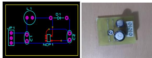
Fig. 3 Raspberry Pi W system power adapter using NCP 1402: schematic, PCB and result.
