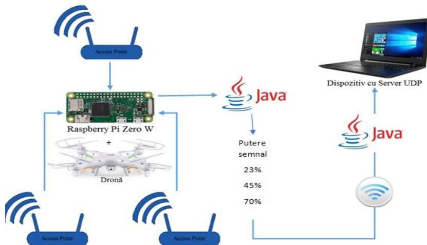
Fig. 4 System components and the communicating server and client applications
