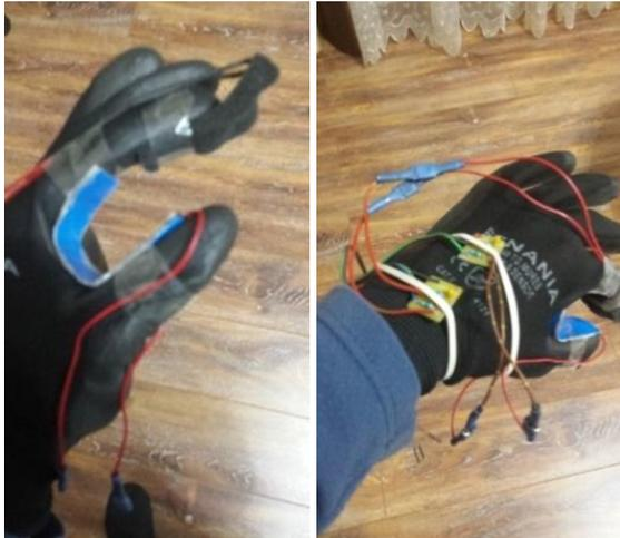
Fig. 10 The glove with attached sensors and the step response circuit. The bending sensors are placed on the fingers inside area
