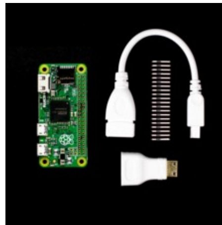
Fig.4 The default starter kit for Raspberry Pi Zero
